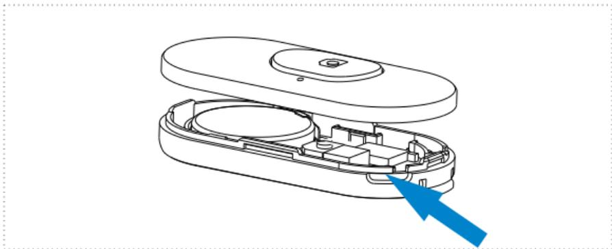
3. Remove the old battery, and dispose of according to local regulations. **Do not dispose of with regular household waste.**
