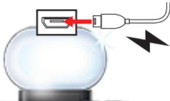
Plug the USB (larger) connector into a USB power source, such as the USB port on a computer or a 5V USB wall adapter (not included).
