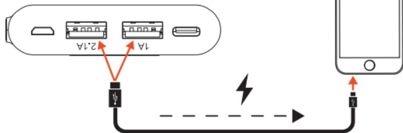
The power bank can power or charge any device that is powered or charged by a USB cable or USB connector. Just plug the USB connector into either of the power bank's USB output ports.
