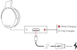
The LED indicator will turn solid RED while charging and turn OFF when fully charged. On low power a tone will be heard, indicating that the headphones should
