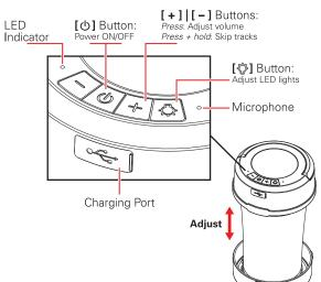
Undo the rubber seal covering the charging port, and plug the small connector of the supplied charging cable into the charging port. Plug the large connector into a USB power port or a **5V USB adapter** (not included) and plug into a wall outlet.
