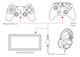
Insert the headphone connector into the headphone jack on your controller. Insert the USB connector into a **5V USB** power source to use the headset lights.
