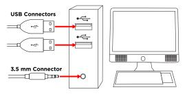
The keyboard, mouse and headphones should not require any special installation or software to connect to your computer. Your computer should automatically detect and install them, and their lights should automatically
