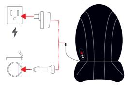
Warning: Do not plug the attached USB connector into your car's built-in USB power port. This can damage the device or the USB port. Use with an adapter that plugs into the cigarette lighter ONLY.
