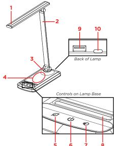
2. Plug the small connector of the included charging cable into the power port on the back of the lamp, as shown in the diagram below. **∮**USB **Power** Back of 3. Plug the large connector into a USB power sou
