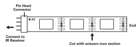
Using a pair of scissors, carefully clip along the dotted cut line of the LED strip. Do NOT sever or cut the copper contacts on either side of the dotted cut line.
