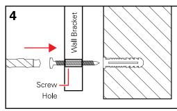
4. Place the wall brackets back on the wall and carefully drill them into the anchors using the mounting screws.
