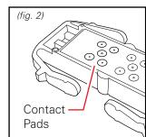
When the bracket connectors are clipped into place, power is carried through the whole system. If one connector is not properly connected then there will be no power to the rest of the system.
