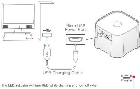
The LED indicator will turn RED while charging and turn off when fully charged. On low power, a tone will be heard indicating that the speaker needs to be recharged.
