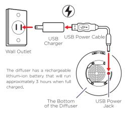
The LED indicator will flash when the battery needs to be recharged. It takes 7-8 hours to fully recharge the diffuser.
