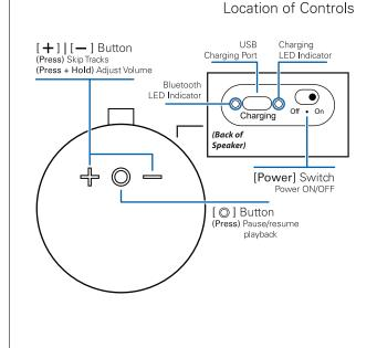
Charging the Speaker Attach the small connector of the supplied USB charging cable to the USB charging port on speaker. Attach the large connector to the USB port on a computer, a USB charging device, or a 5V USB adapter (not included) and plug into a wall socket.
